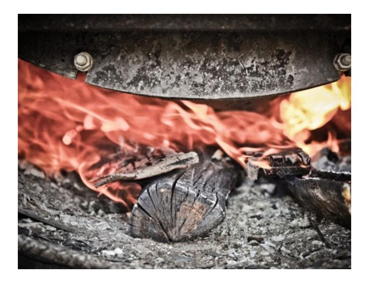
Once in the firebox this highly flammable gas burns and raises the temperature still further. After this point has been reached the machine is self fueling and requires only small adjustments to the firebox door and a bleed valve on a retort chamber vent to control gas supply to the firebox, and therefore temperature.
