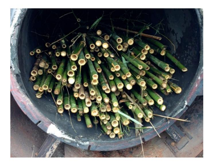
This method of production also allows unusual loads to be converted to charcoal. We have proved the Exeter Retort with some odd materials. We have converted reed, bamboo and even bone with our machine. None of these feedstocks can be processed in the traditional way.
