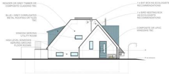
PROPOSED South-west elevation (rear) 1:100
