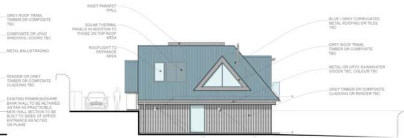
PROPOSED South-east elevation (field side) 1:100
