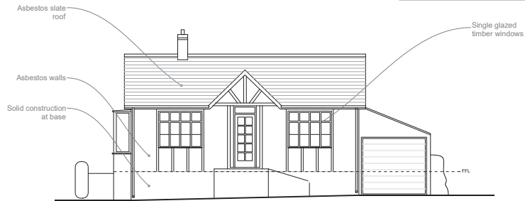
EXISTING Northeast Elevation (front) 1:100
