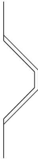
POND - LINED WITH 150mm COMPACTED CLAY SUBSOIL
