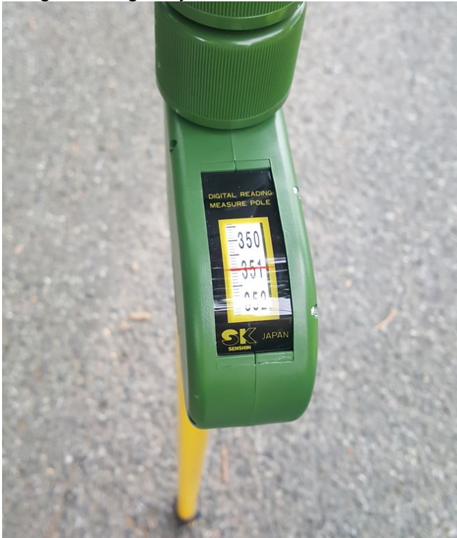
Image 6 – Highway clearance measurement
